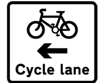
Cycle lane on road at junction ahead or cycle track crossing road
